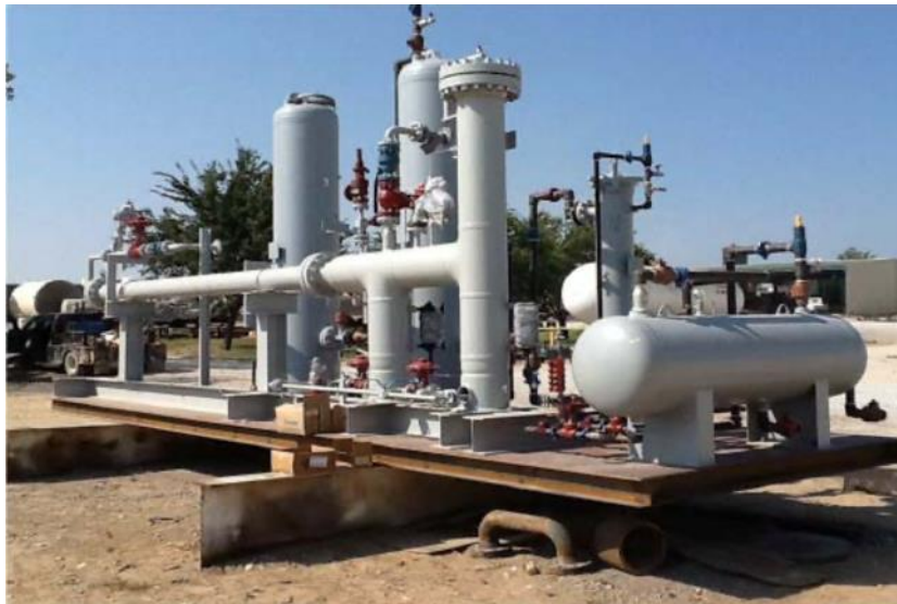
A standard package WSCE MiniLNG-1 at a remote natural gas well site. The capacity is 4,000 US gallons (350,000 ft 3 /d)
